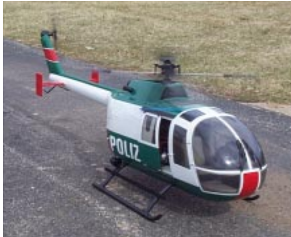
Slim Helson's B0-105. Fuselage kit: Vario Mechanics: Futura SE Engine: Webra 75 Weight: 13 lbs.. Blades. NHP 710's Radio: JR
